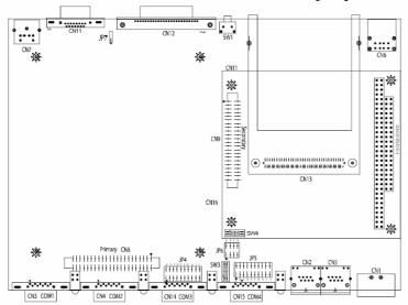
Figure A.1: UNO-2170 connector and jumper locations (front-side)
